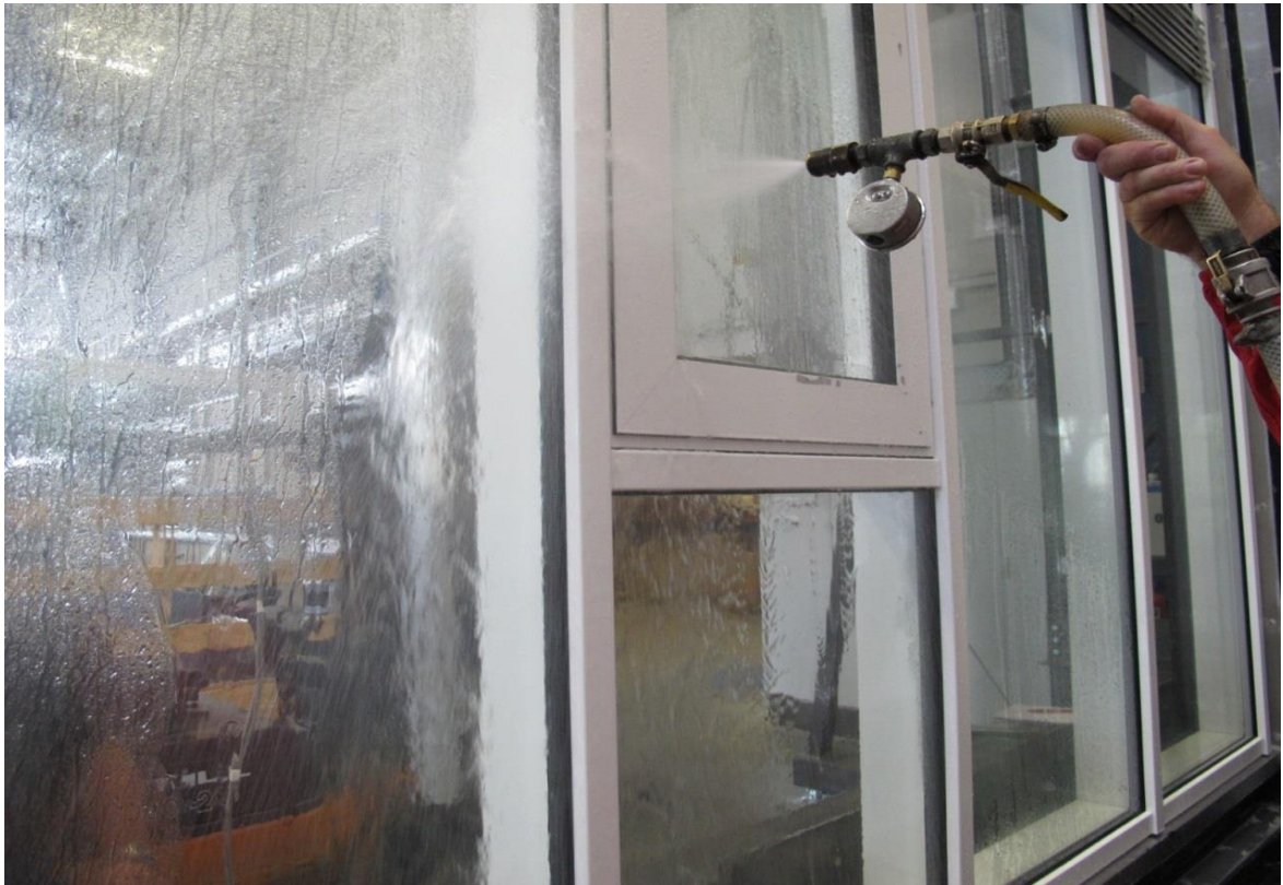
Hose spray test
